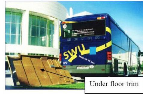
Figure 8: Automotive exterior components made from flax fiber reinforced composites
