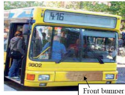
Figure 8: Automotive exterior components made from flax fiber reinforced composites
