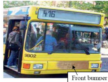
Figure 8: Automotive exterior components made from flax fiber reinforced composites
