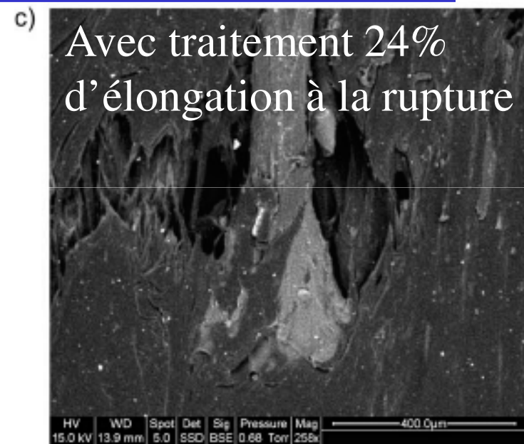
Fig. 5. SEM micrographs for an irradiated (25 kGy) 50/50 w/w% rHDPE/GTR blend under tensile deformation: (a) 0% strain, (b) 22% strain, and (c) 24% strain.
